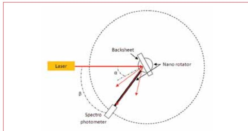
**Figure 6. Set-up used to measure the angular dependence of the backsheets. The laser is placed in a fixed position, and the backsheet is put on a rotating base. The base can be rotated from  $\alpha = 0$  to  $90^\circ$ , where  $\alpha$  is the angle between the laser beam and the perpendicular to the backsheet; this angle is kept fixed during a measurement.  $\beta$  is the angle between the laser beam and the spectro-photometer, and can vary from  $0$  to  $360^\circ$ .**
