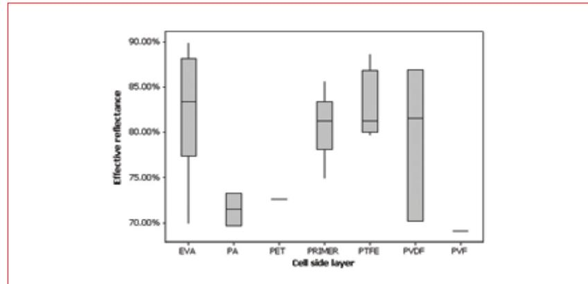
**Figure 5. Effective global reflectance of the backsheets analysed. (Cell-side layers: EVA – ethylene vinyl acetate; PA – polyamide; PET – polyethylene terephthalate; PTFE – polytetrafluoroethylene; PVDF – polyvinylidene fluoride; PVF – polyvinyl fluoride.)**
