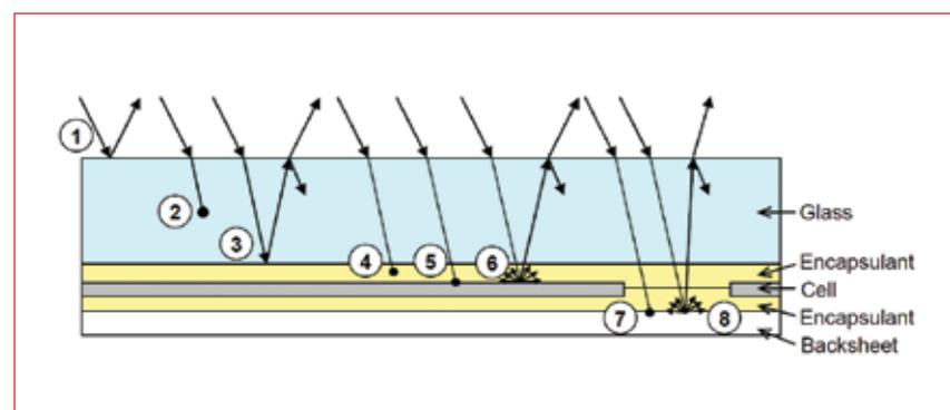
Figure 1. Cross-sectional diagram of a conventional PV module (to scale), and optical loss mechanisms [1].
