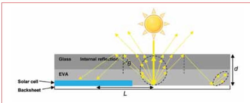
Figure 2. Cross section of a conventional PV module.
