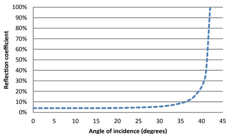
Figure 3. Reflection coefficient as a function of the angle of incidence for a non-polarized ray of light at the glass–air interface.
