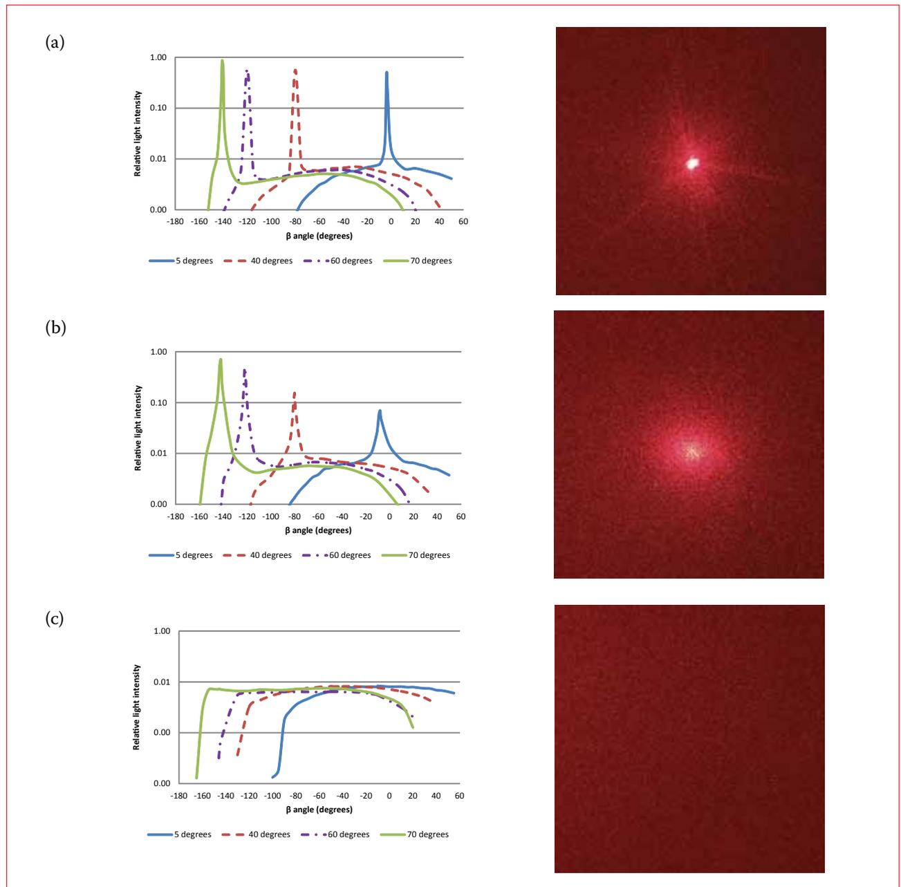
Figure 7. Angular distribution profiles for a backsheet with (a) high specular reflection (group A); (b) medium specular reflection (group B), and (c) low specular reflection (group C). The photograph on the right in each case shows the reflected light for an incident angle of 5°.
